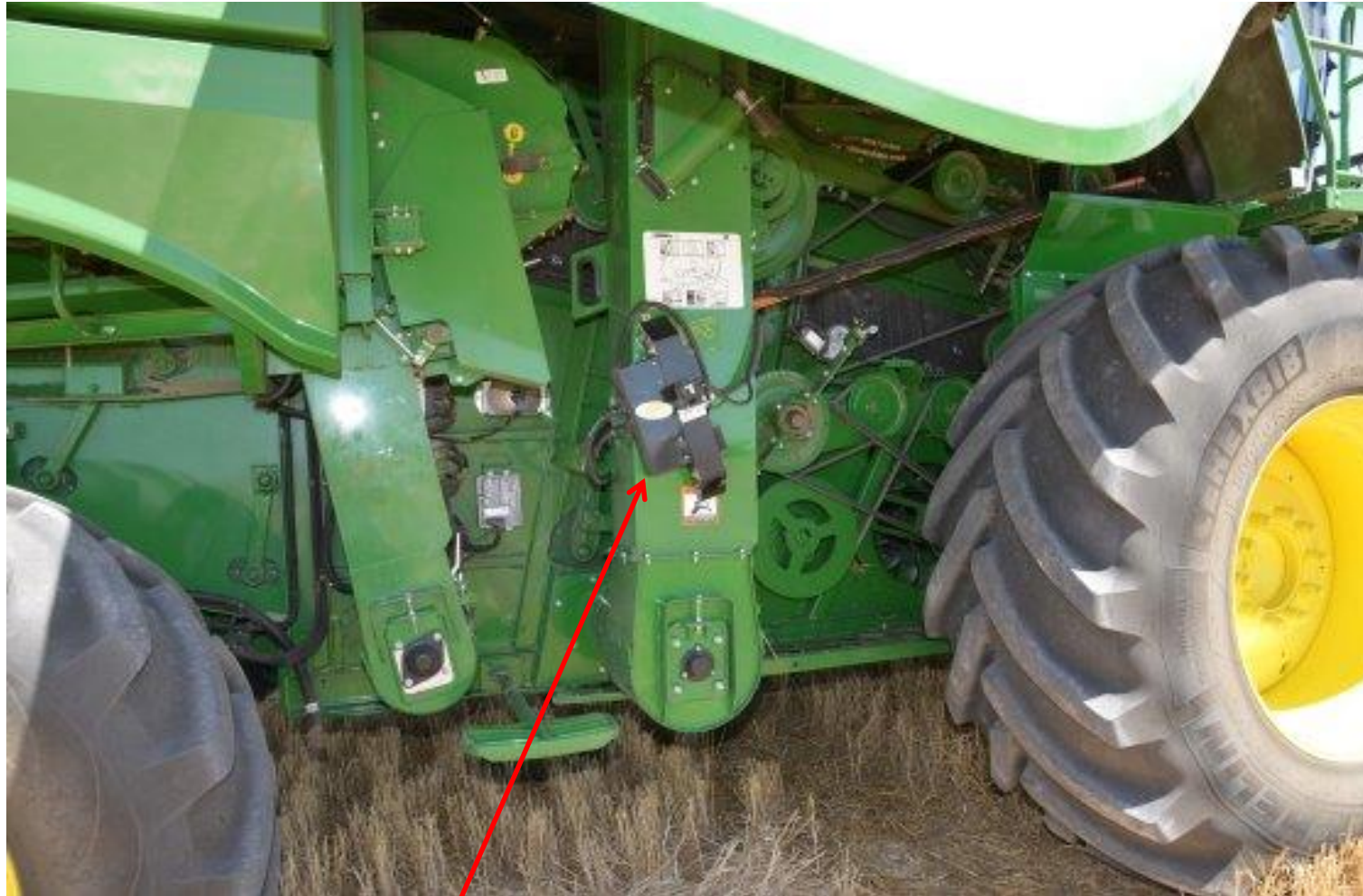
Protein sensor mounted on the clean grain elevator
