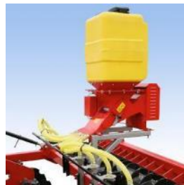
Schematic of a variable rate seeder: this solution allows seed mixing, specific seed selection, and the variation of the amount of seeds per unit.
