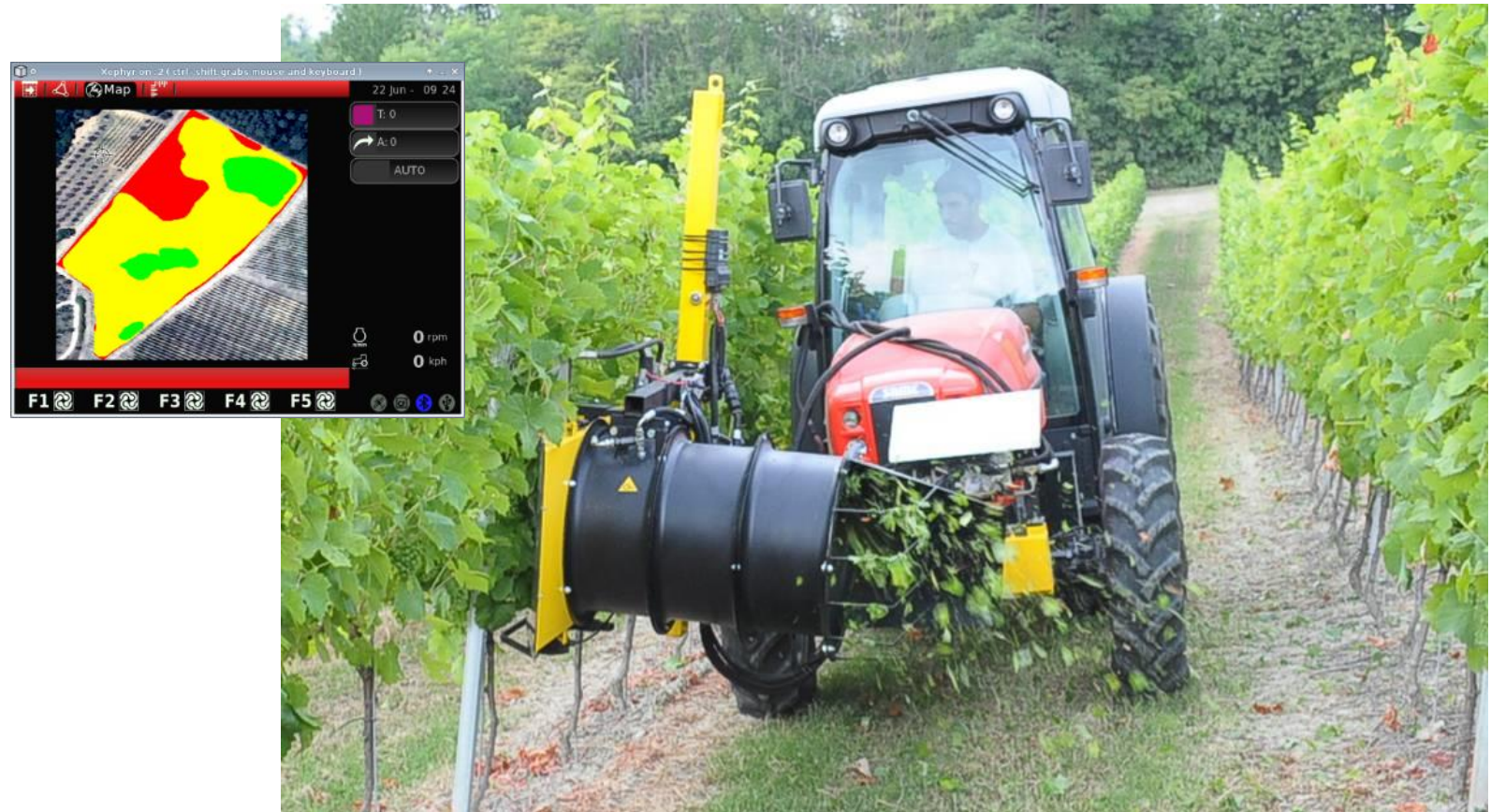
Vineyard leaf stripper with automatic tracking treating the canopy
